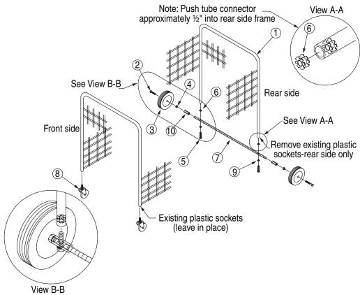
To convert the standard model Ball Storage Cart to the "all-terrain" style, follow the instructions provided below carefully. Tools required: Small Hammer (1); Flat Blade Standard Screwdriver (1); Small Adjustable Wrench (1).
